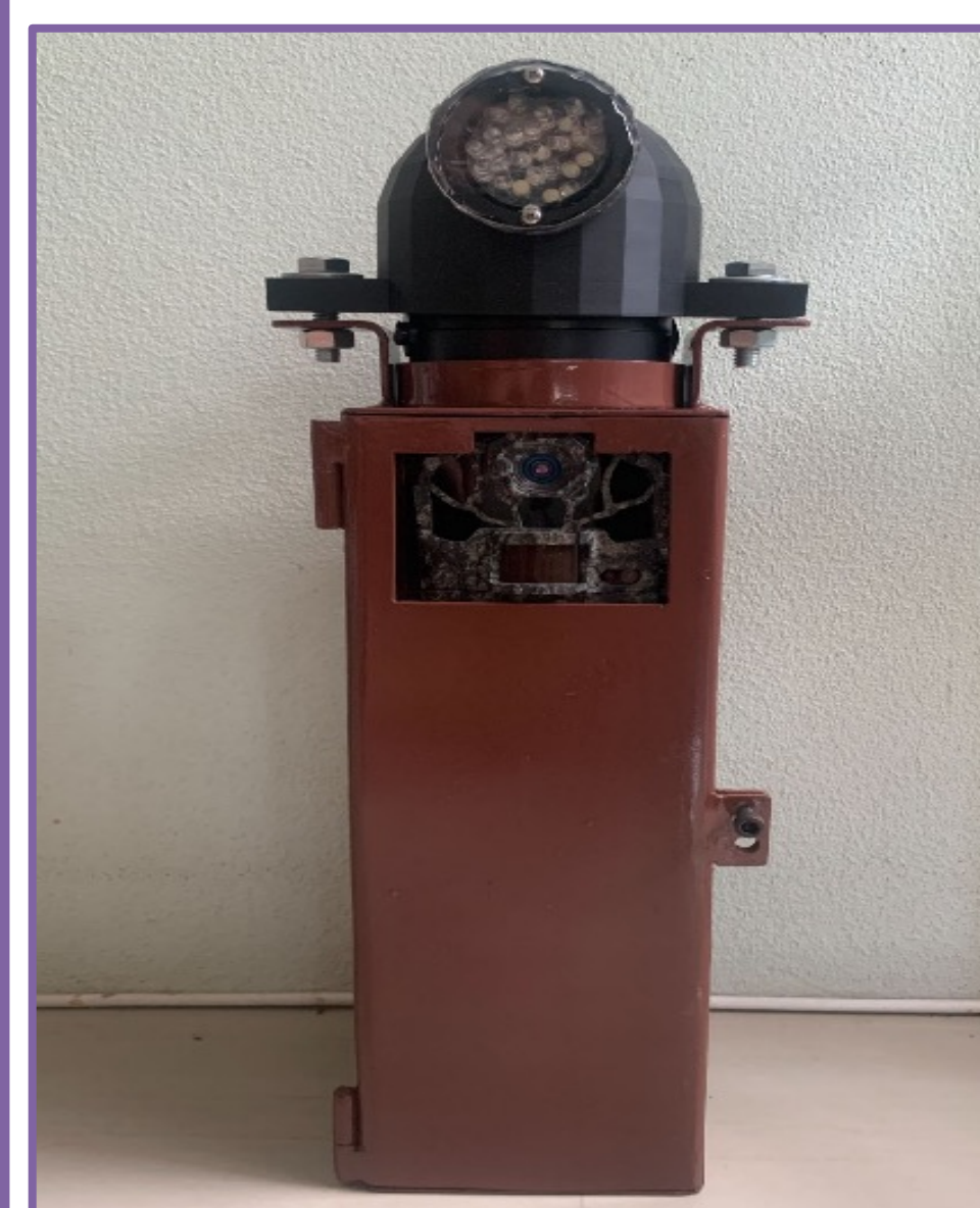
Light-emitting device and front facing camera, placed inside a brown metal mounting box.
